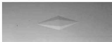
Figure 4: Ice crystal formation in a glass capillary in the presence of winter flounder type I antifreeze protein. The shape reflects the binding of winter flounder AP to the pyramidal \{20\bar{2}1\} plane of ice. Picture from [3].
