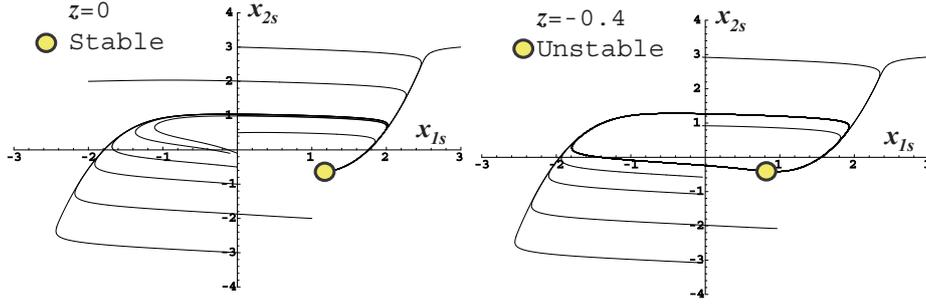
Figure 3:  $x_1(t), x_2(t)$  trajectories for different starting points (open ends of the trajectories). In case of a stable stationary point, all the trajectories come to rest at the stationary point whereas in case of an unstable stationary point the system begins a cyclic motion, regardless of its starting point.
