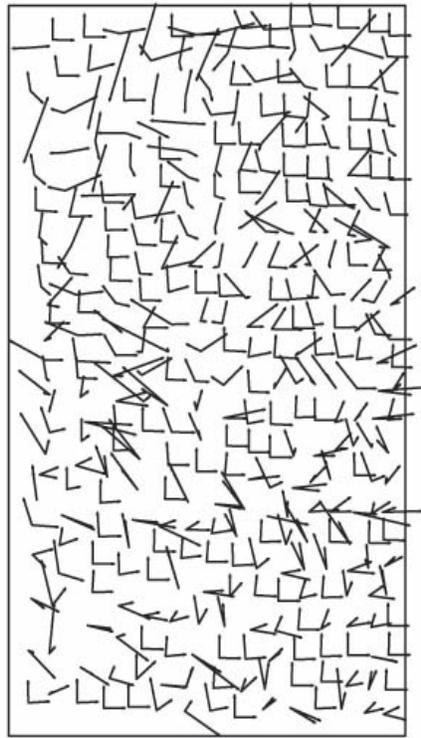
**Abb. 13.9:** Result of the same simulation as in Fig. 13.1-13.3, obtained after 10,000 learning steps, but without lateral interaction between the array variables  $\mathbf{A}_r$ , i.e., with  $h'_{rs} = \delta_{rs}$ . In this case, the desired convergence is only achieved for a fraction of all end effector configurations. This illustrates the important contribution of lateral interaction to a robust convergence behavior of the system.
