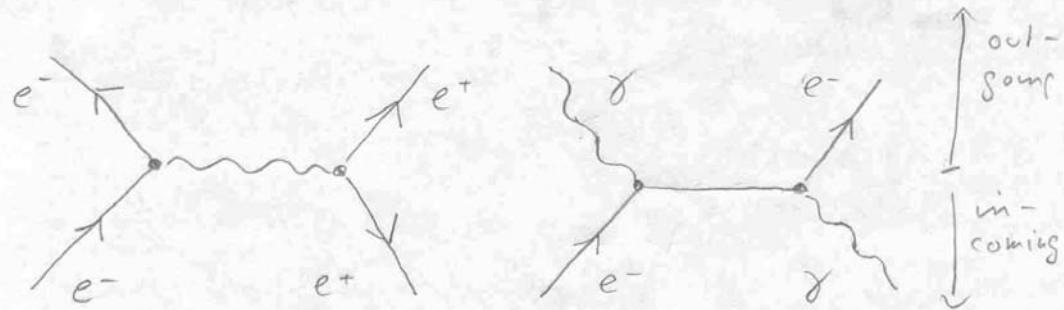
For a particle ( $e^-, \mu^-, \tau^-$ ), the arrow points to the vertex when it is incoming, away from it, when it is outgoing; for an antiparticle ( $e^+, \mu^+, \tau^+$ ), it is the opposite.
