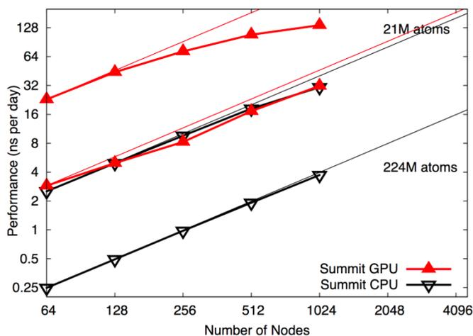
Figure 5: NAMD strong scaling results comparing stochastic velocity rescaling to Langevin damping.
