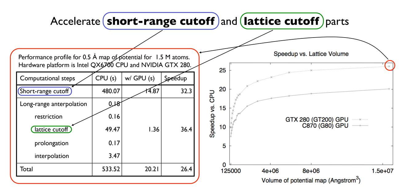
Multilevel summation of electrostatic potentials using graphics processing units. D. Hardy, J. Stone, K. Schulten. J. Parallel Computing, 35:164-177, 2009.
