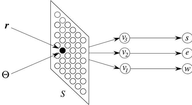
Figure 1: The basic network used to control movement.  $w, e$  and  $s$ , refer to the joint wrist, elbow and shoulder joints of the arm respectively. Definitions of all other quantities may be found in the text.
