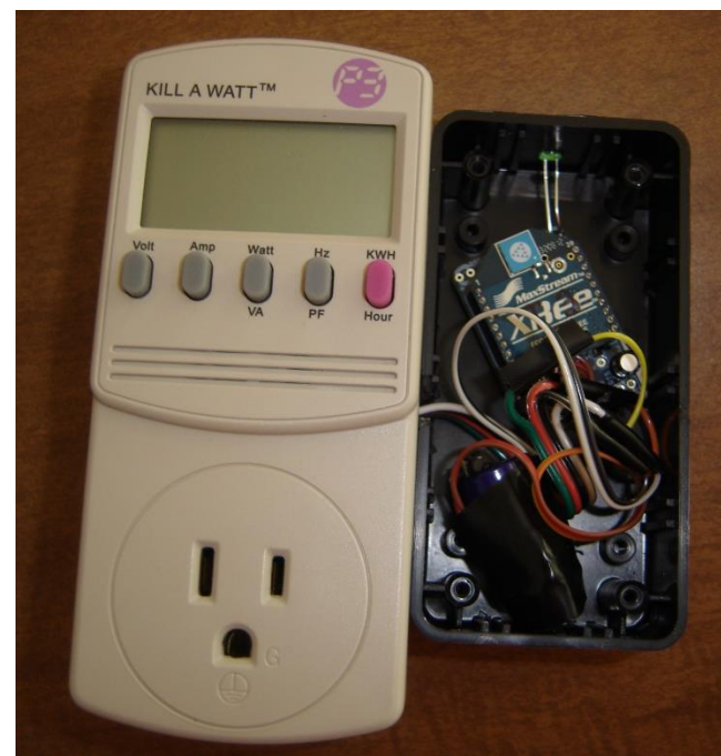
NCSA Tweet-a-watt power monitoring device
