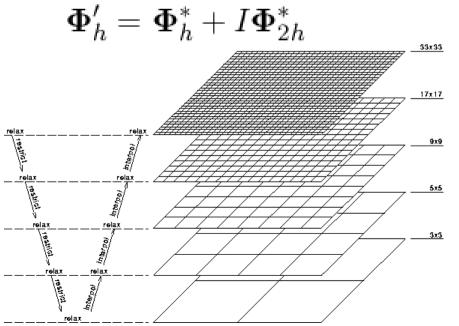
Interpolate coarse solution onto finer grid and add to approximate fine solution
