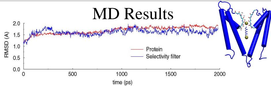
RMS deviations for the KcsA protein and its selectivity filer indicate that the protein is stable during the simulation with the selectivity filter the most stable part of the system.
