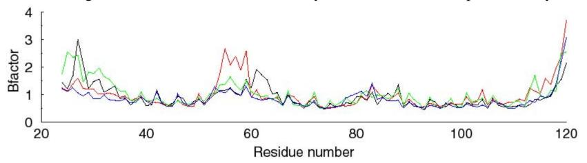
Temperature factors for individual residues in the four monomers of the KcsA channel protein indicate that the most flexible parts of the protein are the N and C terminal ends, residues 52-60 and residues 84-90. Residues 74-80 in the selectivity filter have low temperature factors and are very stable during the simulation.
