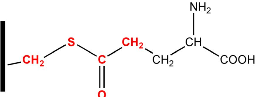
HG1 deleted from CYS and the charge was moved to SG ( $-0.23 + 0.16 = 0.07$ ) so that the SG charge becomes 0.07 in final compound and the group remains neutral.
