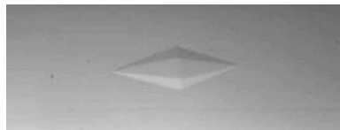
Figure 4: Ice crystal formation in a glass capillary in the presence of winter flounder type I antifreeze protein. The shape reflects the binding of winter flounder AP to the pyramidal \{20\bar{2}1\} plane of ice. Picture from [4].
