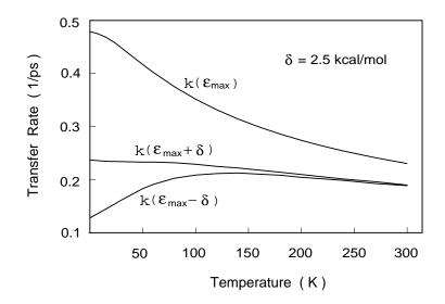
Figure 3: 1 Comparison of the temperature dependence of the maximum transfer rate of  $k(\epsilon_m)$  and off-maximum value  $k(\epsilon_{max} \pm \delta)$ , where  $\delta = 2.5$  kcal/mol.  $k(\epsilon_{max}, T)$  represents the fastest transfer rate of the system, the rates  $k(\epsilon_{max} \pm \delta, T)$  are slower since their E-values deviate from the optimal value  $\epsilon_{max}$ . From [3].
