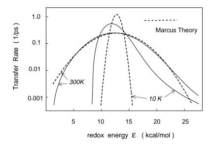
Figure 2: Comparison of electron transfer rates  $k(\epsilon, T)$  shown as a function of  $\epsilon$  evaluated in the framework of the spin-boson model (solid lines) and by Marcus theory (dashed lines) at temperatures 10 K and 300 K. The functions are centered approximately around  $\epsilon_m$ . From [3].
