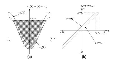
Figure 9.2: (a) Relative position of the two energy sub-bands  $\epsilon_{\alpha}(k)$  and  $\epsilon_{\beta}(k)$  for  $\Delta = n_{\alpha} - n_{\beta} > 0$ . The shaded areas represent the filled portions of these bands by electrons. (b) Graphical definition of the limiting energies  $\epsilon_{\alpha}$  and  $\epsilon_{\beta}$ .
