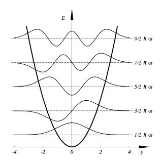
Figure 2.2: Stationary states  $\phi_n(y)$  of the harmonic oscillator for n = 0, 1, 2, 3, 4.
