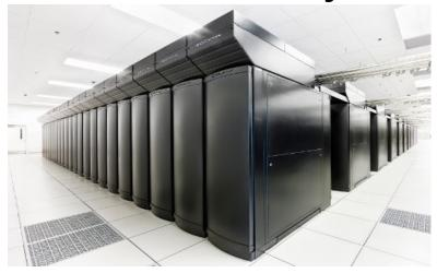
NCSA Blue Waters Hybrid Cray XE6 / XK7 Supercomputer 22,640 XE6 CPU nodes
