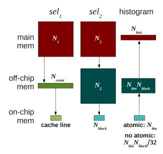
Figure 2: This illustration depicts the way our implementation of RDF histogramming makes use of the memory hierarchy of the GPU to store geometric  $(sel_1 \text{ and } sel_2)$  and histogram data. Main memory (off-GPU) is shaded red. Constant memory and the constant cache are shaded dark and light green respectively. Global and shared memory are shaded dark and light blue respectively. The number of atoms or histogram bins stored at each level of memory is marked on each piece of memory.
