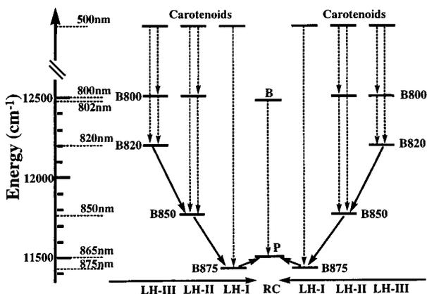
FIG. 2. Energy levels of the electronic excitations in the PSU of BChl *a* containing purple bacteria. The diagram illustrates a funneling of excitation energy toward the photosynthetic RC. The dashed lines indicate (vertical) intracomplex excitation transfer, and the solid lines (diagonal) indicate intercomplex excitation transfer. LH-I exists in all purple bacteria; LH-II exists in most species; LH-III arises in certain species only.
