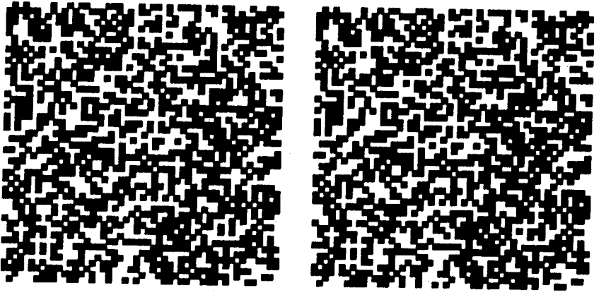
Figure 17. Julesz pattern 23 with 50% black dots. This random-dot stereogram of 50 \times 50 pixels is generated by copying the right image from the left one, shifting a square-shaped region of 30 \times 30 pixels slightly to the left and filling the gap caused by the shift with a new random pattern.
